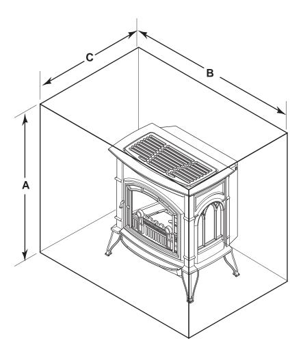
Figure 6 - Placing Stove in Alcove
